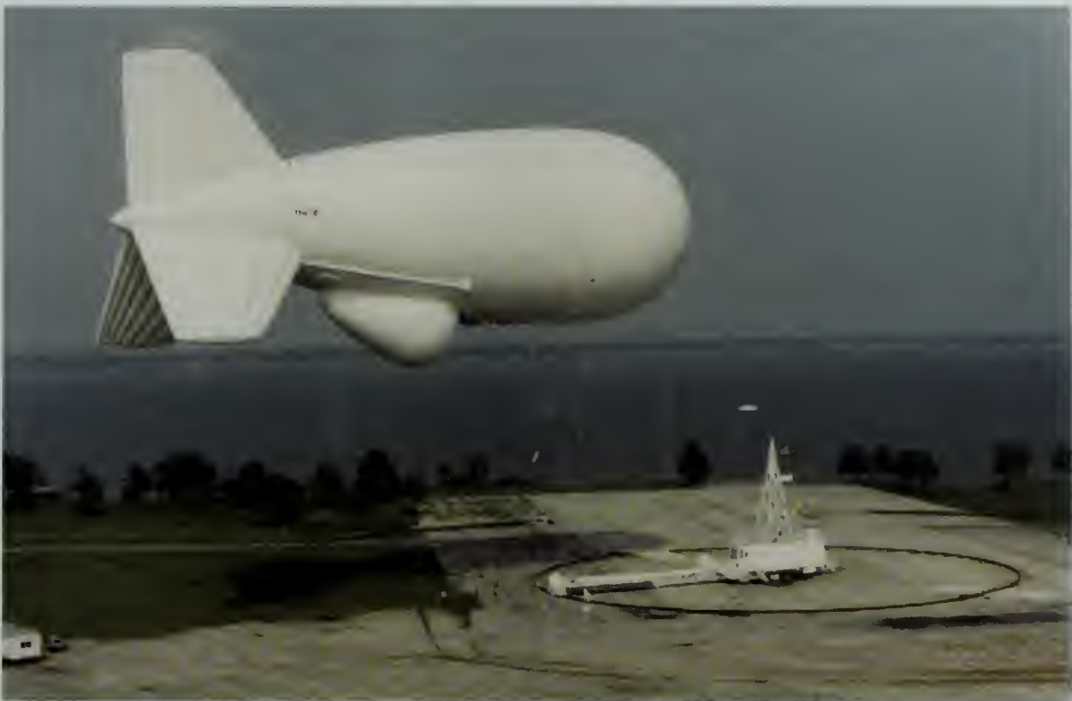
Fig. 6-12. The cost effective Joint Land Attack Cruise Missile Defense Elevated Netted Sensor System employs an aerostat, a tethered helium-filled blimp, outfitted with radar and communications equipment that operates at altitudes between 10,000 and 15,000 feet to see over the horizon.
